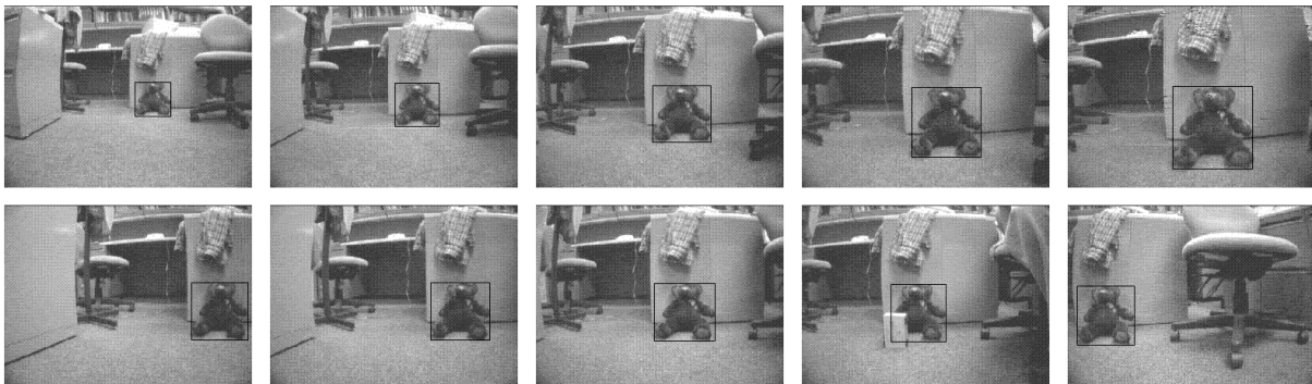
Figure 4. Tracking of the bear images in a frame sequence. Pictures in the first and second rows were taken when the robot was “going forward” and “turning right”, respectively
