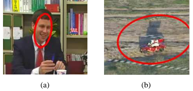
Fig. 2. With the moment-size relationship of Eq. (6), CamShift succeeds in tracking a man’s face (a); while the scale adaptation fails when tracking a red car in field (b).
