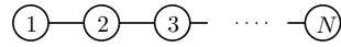
Fig. 1. A linear network. The numbers in the circles are indices of nodes.
