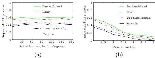
Figure 3: Repeatability rate for image rotation (a) and scale change (b) ( $\epsilon=1$ )
