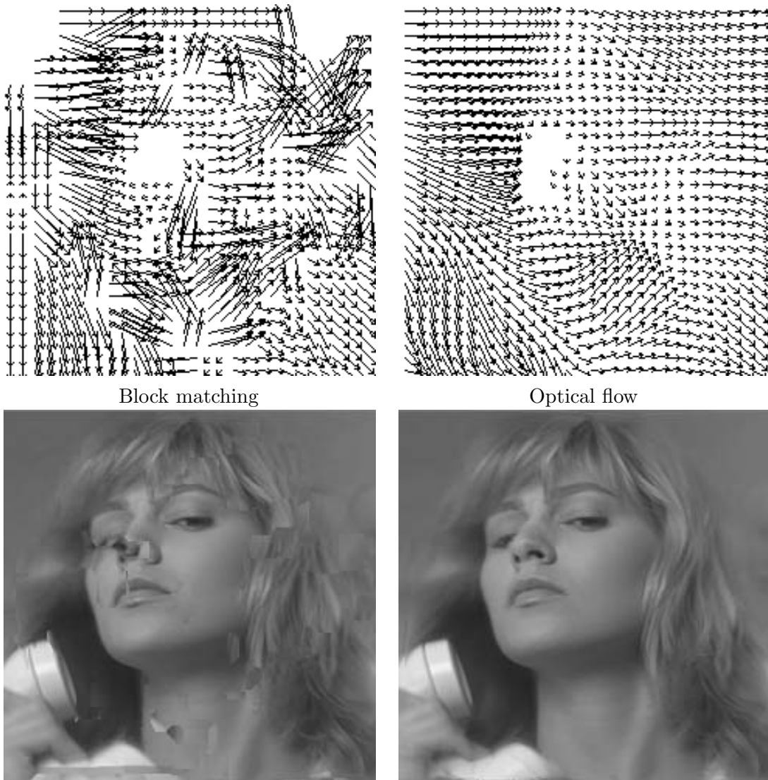
Figure 13: Reconstruction of Frame 47 from Frames 46 and 48 [13]
