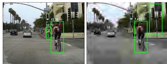
Fig. 1. Detection results of the state of the art pedestrian detector, the Fastest Pedestrian Detector in the West (FPDW) [1] are shown in green bounding boxes. The left is an uncompressed frame and the right is a JPEG 2000 compressed frame at compression ratio of 1000.
