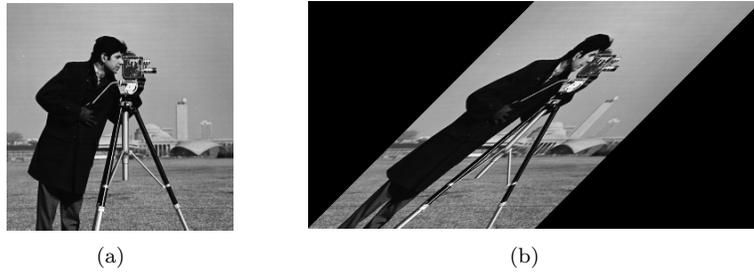
**Figure 6.** Example of a resampling operation that is used effectively as a rotation operation for the DFB decomposition. (a) The “cameraman” image. (b) The “cameraman” image after being resampled.
