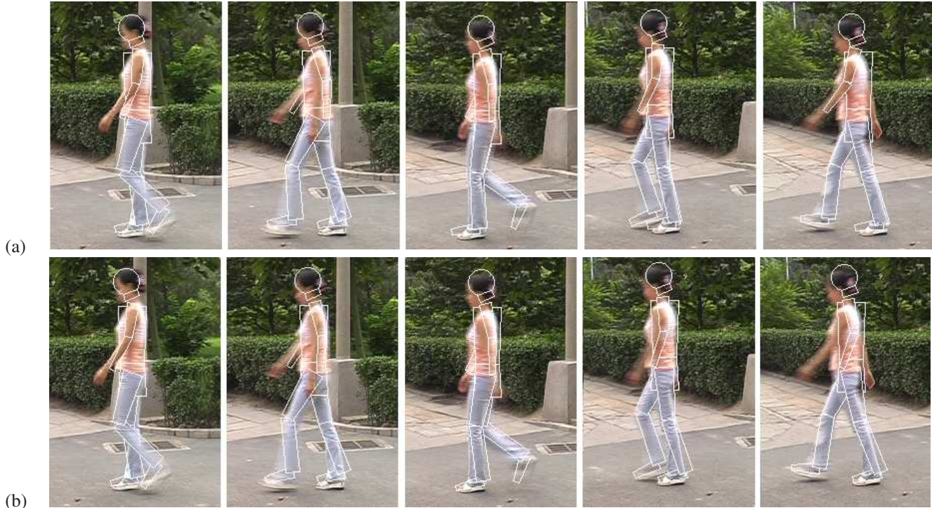
Figure 3. Articulated tracking results: compared with the fusion by fixed weight. (a): Results of fusion framework with dynamic fusion weights (The dynamic fusion weights are shown in figure 4(a) ); (b): Results of empirical fusion with fixed weights \alpha = 0.1 .
